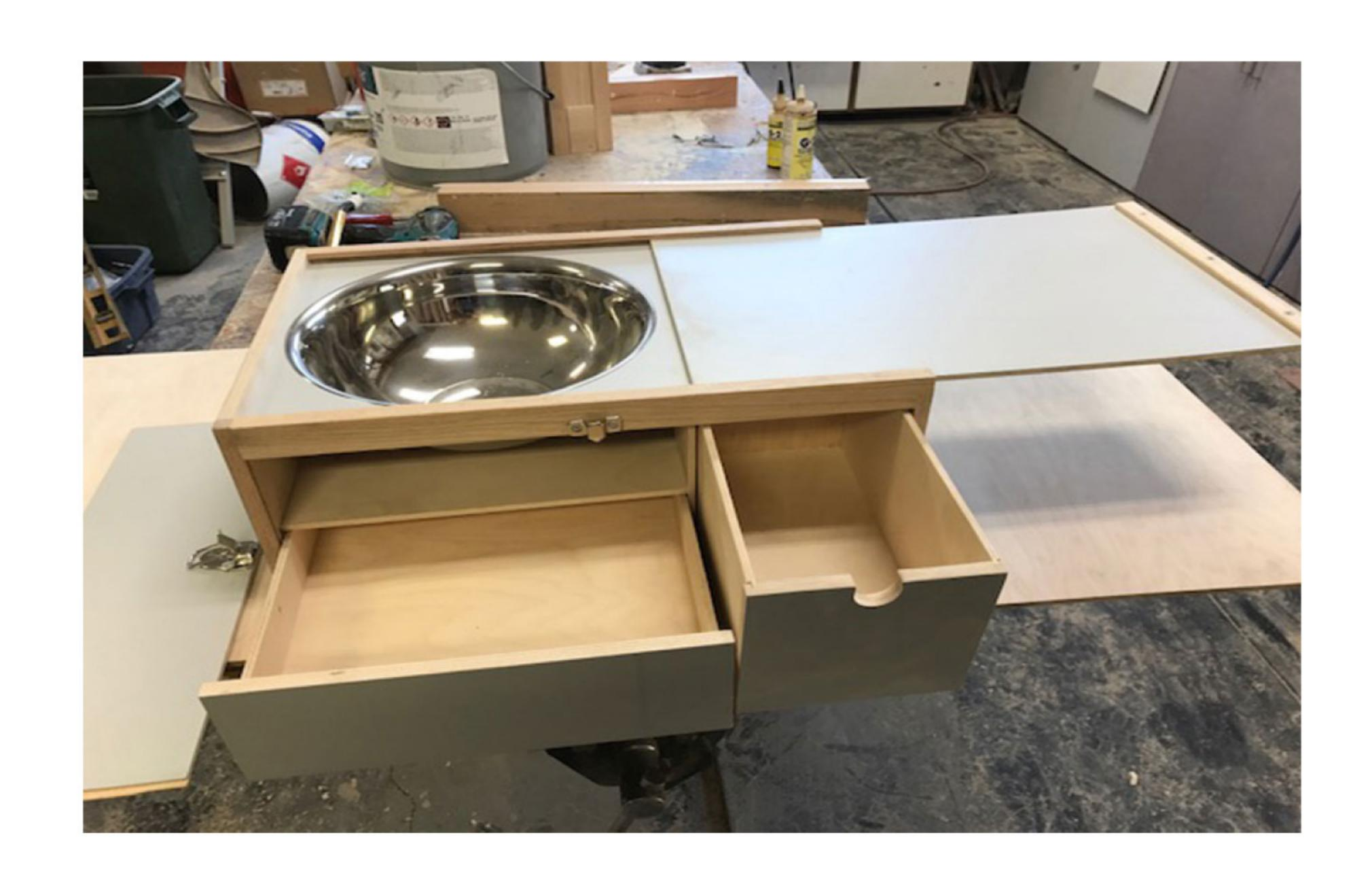
New version is 19.5"x 13 ¼"x 7.5": built of high density Baltic birch plywood and Surfaced with plastic laminates, hardwood trims, and wax sealants applied.
